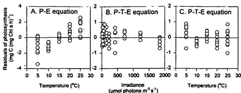
Fig. 6. Representative plots of residuals from non-linear regression analysis of photosynthetic data as a function of the independent variables temperature and irradiance. (A) Residuals from running the Platt *et al.* (1980) equation; (B) and (C) residuals from running the *P-T-E* equation (data for total community, experiment Lake Kayouk I).
