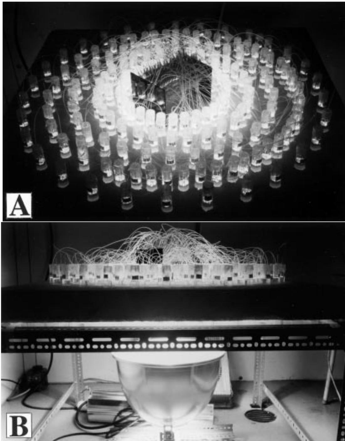
*Figure 1.* View from above (A) and the side (B) of the experimental setup with the lamp, the five irradiance conditions and the air bubbling system.
