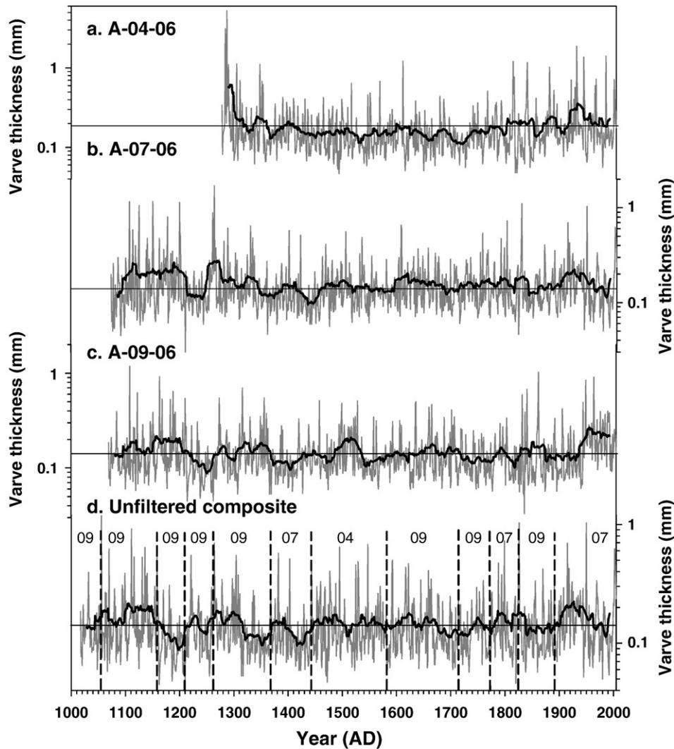
**Figure 4.** Unfiltered varve-thickness records from cores (a) A-04-06, (b) A-07-06, and (c) A-09-06 and (d) the unfiltered composite varve-thickness record that incorporates varve-thickness values from all three cores (indicated by 04, 07, and 09), plotted on a base-10 logarithmic scale. Dashed lines indicate marker beds, thin black lines indicate mean varve-thickness for each core and thick black lines indicate 25-yr unweighted moving means.
