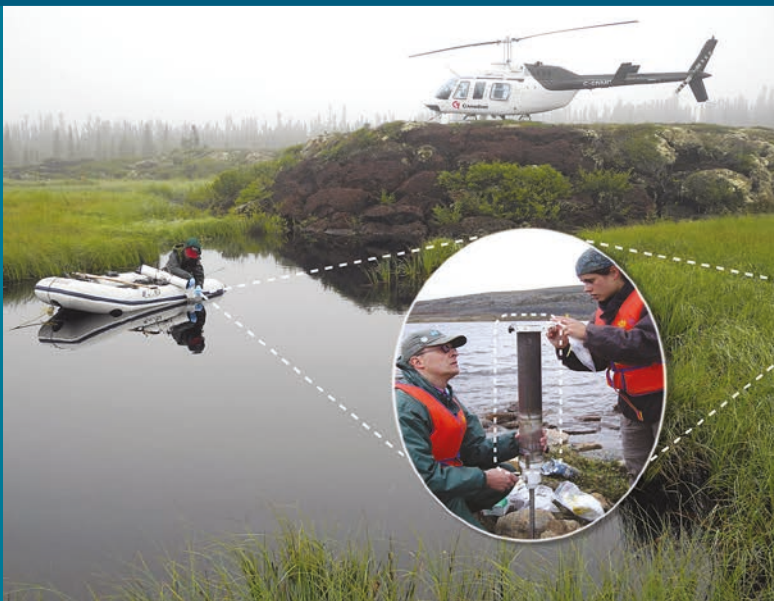
Figure 6.5 Left: paleolimnological analysis of a sediment core, for example from a thaw pond pond formed by a degrading palsa (permafrost mound) near the CEN Whapmagoostui-Kuujuarapik Research Station (•61), sub-Arctic Canada. The core (middle) is split into sections and each section is then dated based on its radiocarbon ( ^{14}\text{C} ) content. The different chemical and biological analyses (right) of these sections then provide information about historical changes in different features of the lake and its surrounding environment. Modified by Hannele Heikkilä-Tuomaala from Berglund and others 1996 (Warwick F. Vincent and Reinhard Pienitz).
