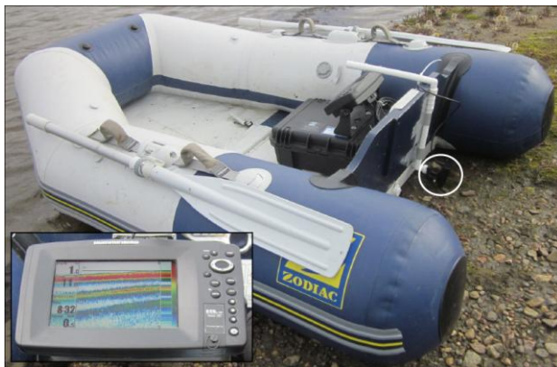
Figure 2. Photographs of the integrated portable GPS-sonar system installed on a small zodiac. The antenna (circled) is fixed outside the zodiac to float at the water surface.
